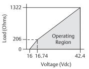
The Field Communicator requires a minimum loop resistance of 250  $\boldsymbol{\Omega}$  for communication.
