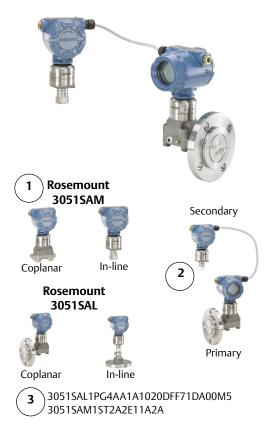
The Rosemount 3051S ERS System is a flexible, 2-wire 4-20 mA HART architecture that calculates differential pressure (DP) electronically using two pressure sensors that are linked together with a non-proprietary electrical wire.
