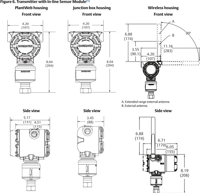
Figure 6. Transmitter with In-line Sensor Module<sup>(1)</sup>
