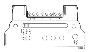
Fig. 3. Q7130A terminals and adjustments.
