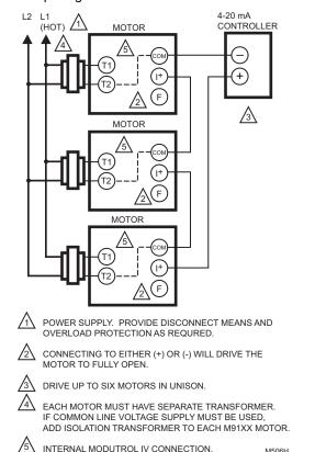
Fig. 7. Typical wiring diagram for Q7230A Interface Module and M91XXX Modutrol IV Motor with 4-20 mA controller.
