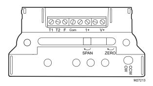
Fig. 5. Q7230A terminals and adjustments.
